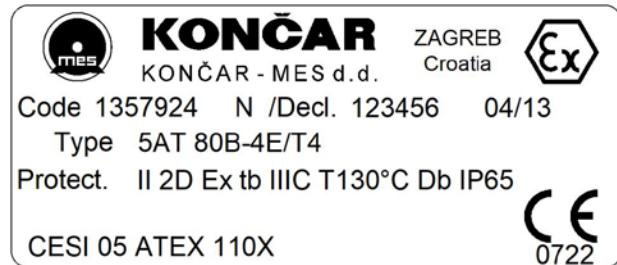
For dust explosion-protected motors the dust explosion protection depends a lot on the local environmental conditions. The motor must be cleaned from deposited dust and other contaminants in regular intervals (depending on conditions), especially the entry openings and air passages of the cooling system as to ensure sufficient air flow to properly cool the motor during operation (check for accumulated dust between the ribs under the protective cover and clean as needed).
