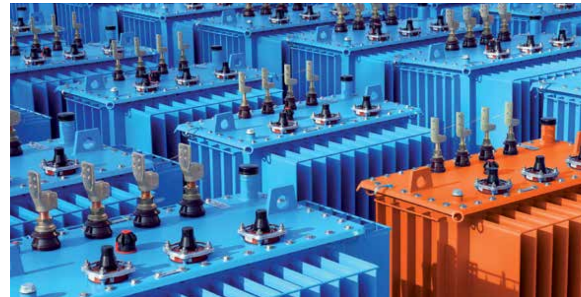
In 2019 KONČAR manufactured 7500 oil-immersed distribution transformers
